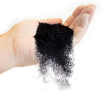
With Genan's cryogenic process technology, liquid nitrogen is used to freeze rubber granulate to a temperature so low that milling results in a fine rubber powder.
